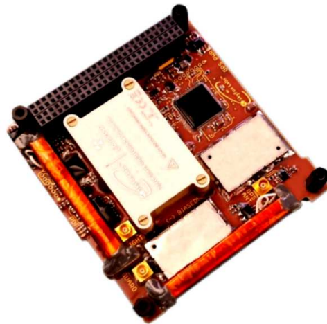
Fig. 1 PC/104+ CubeSat Space Flight & Weather Monitor, Flight Model, Top side view.
