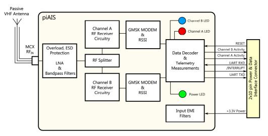
Fig. 3 The piAIS True 2-Channel VHF CubeSat AIS Receiver Block Diagram.
