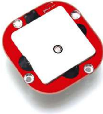
Fig. 4 Engineering Model of the nanoPATCH-L1 unit with red Remove Before Flight finish.
