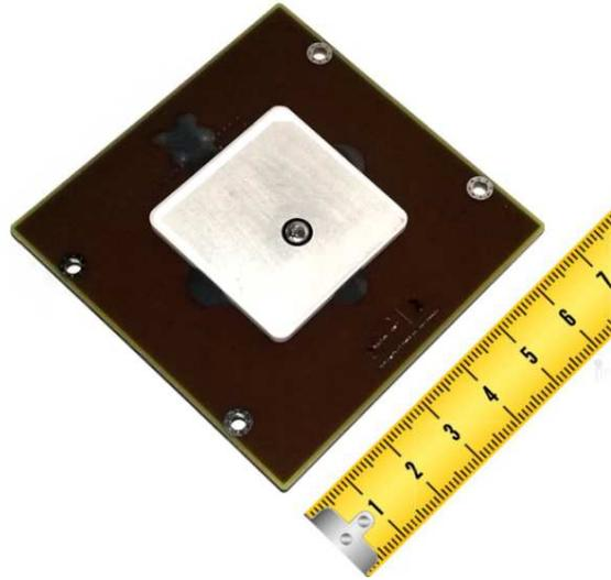
Fig. 1 Mini GPS-L1 Patch Antenna Flight Model.
