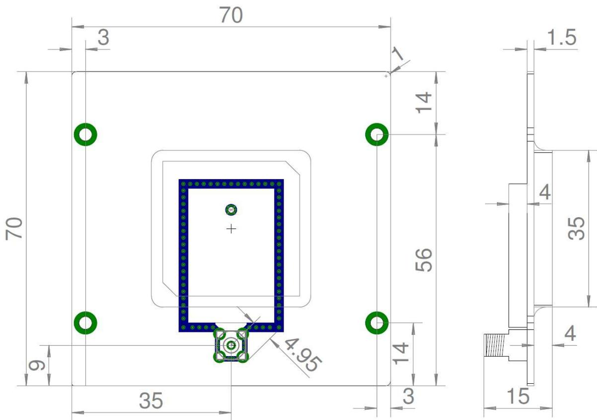
**Fig. 2 mniPATCH-L1 Dimensions drawing.**
