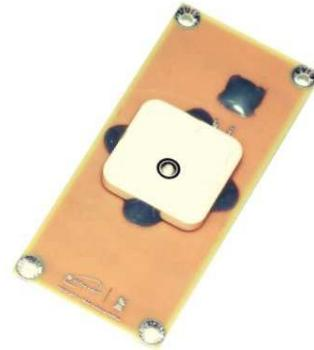
Fig. 1 Micro GPS-L1 Patch Antenna - Flight Model.
